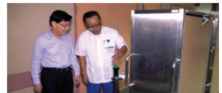
Autonomous delivery robot (HOSPI) delivers medication, specimens, case notes etc. within the hospital
